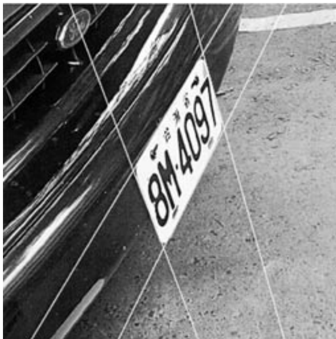
FIG. 9—The position of Fig. 7's vehicle license plate image is processed by X-Y plane rotation.
