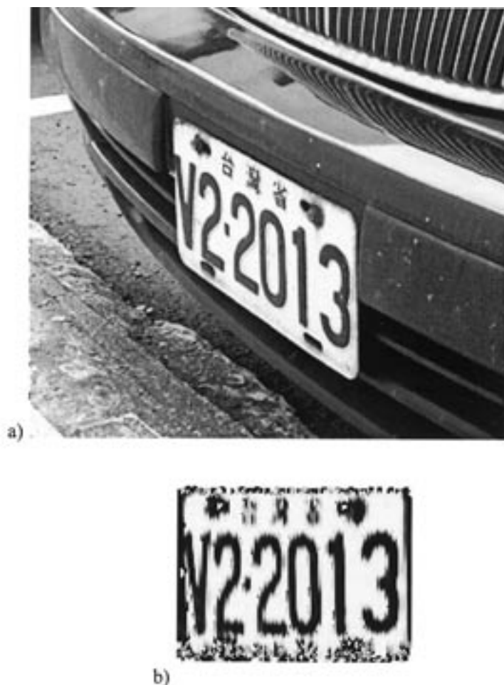
FIG. 14— a) A vehicle license plate image with a different skew distortion angle; b) the normalized result.
